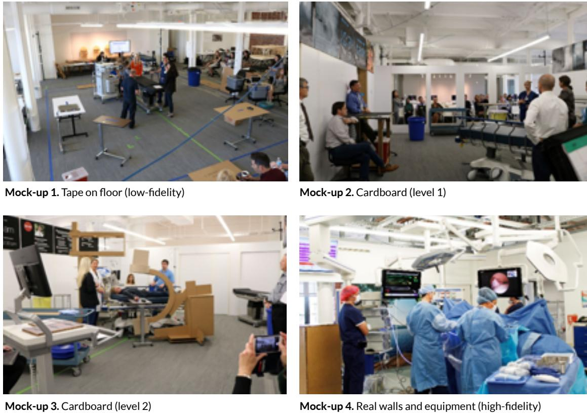
**Figure 2.** Four stages of mock-up development.
